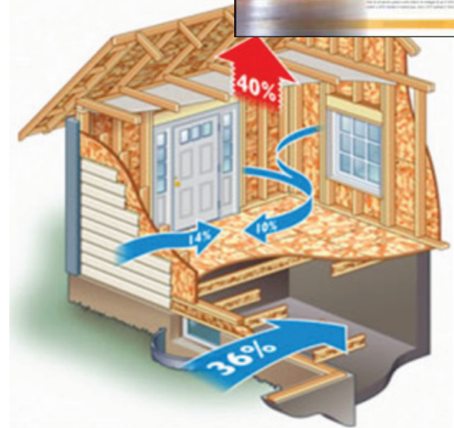
Picture shows typical air leak issues in homes and the increased energy loss
